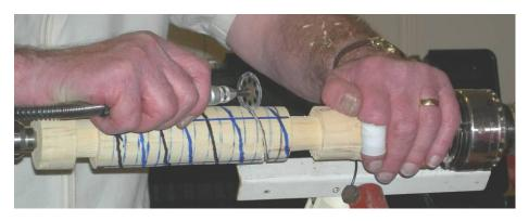
Here, the Multi-tool is used with a Dura-Grit cutter to cut the slots where the troughs will be, following your lines. Here we also see insulating tape being used to stop blood getting on the workpiece. This shouldn't be taken as compulsory equipment, though.
